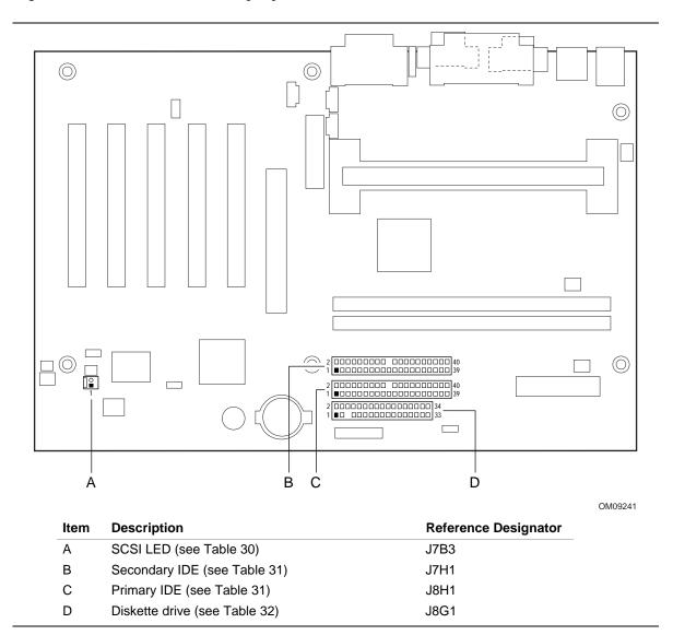
Figure 10. Peripheral Interface and Indicator Connectors
